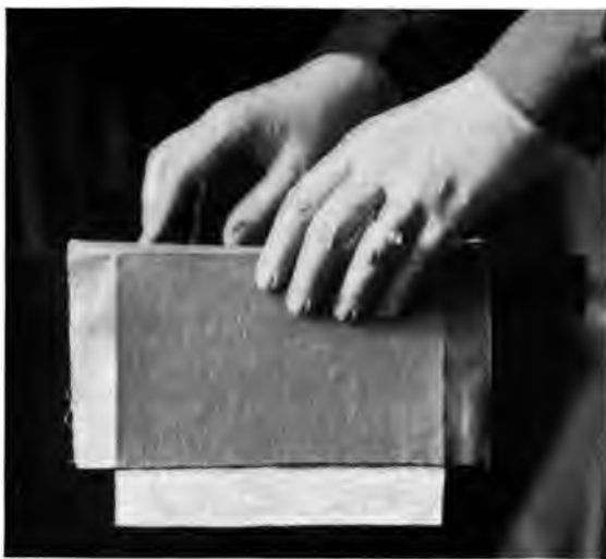
PLATE XXXV. An illustration of the method of covering the outside of the case when no block of wood is available.
