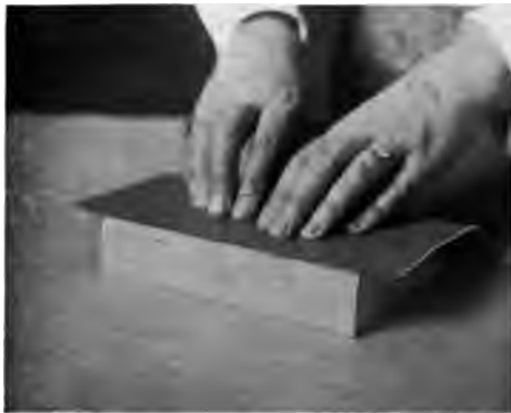
PLATE XXXIV. An illustration of the method of covering the outside of the case when a block of wood is used.
