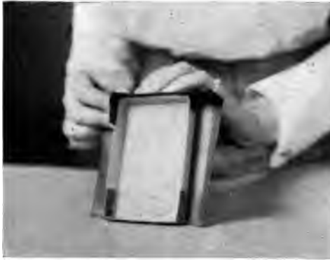
PLATE XXXI. Here the paper is being pasted to the side of the cover.
