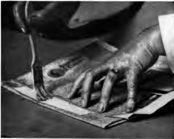
PLATE XLV. Applying paste to the folds of the fly-leaves.
