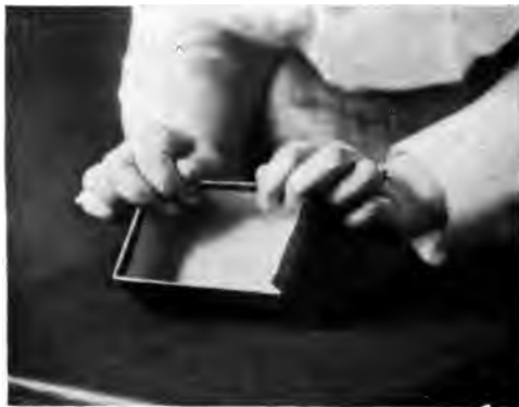
PLATE XXIX. Showing method of pasting the laps to the inside of the box.
