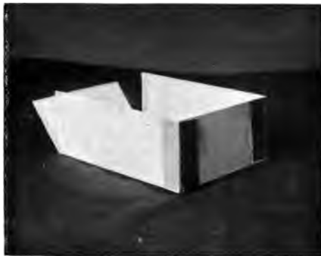
PLATE XXVIII. The box in process of construction showing method of "staying" the corners.
